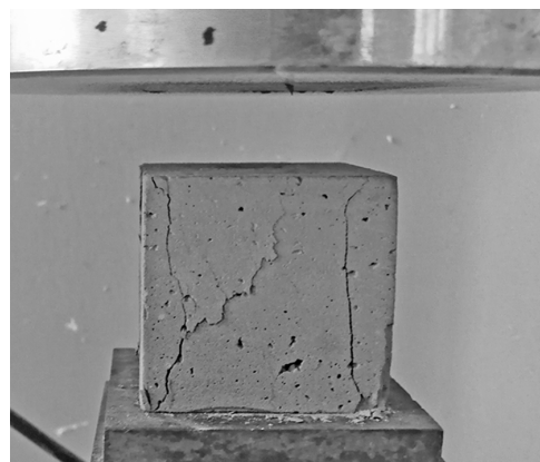
图4 青砖试块受压试验的破坏形态 Fig. 4 Failure morphology of blue brick block under pressure test
